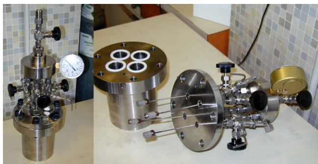
Fig. 1. 4×-parallel stainless steel autoclave with continuous sampling of gas and liquid.
